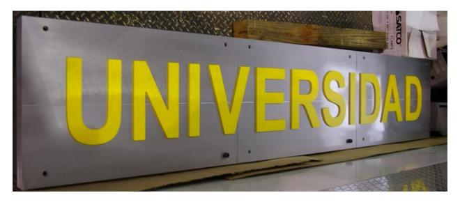
Here's an example of a cabinet sign with routed push-thru letters illuminated from within. Is this sign type potentially prohibited? Obviously, the city is not intending to squelch creative signage, but the definition of cabinets signs as applied in this circumstance is problematic.
